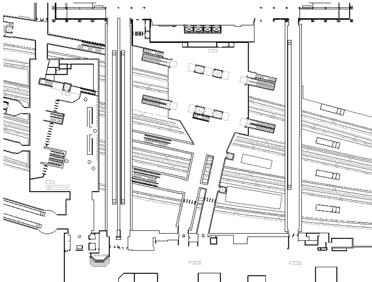
Figure 1. Proposed Development Scheme Design for Gatwick Airport Station including Position of Gatelines
